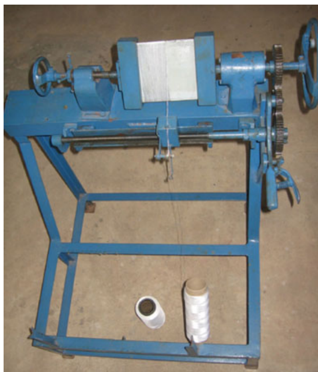
Figure 1 Winding machine developed to mingle and to wind the matrix and the reinforcing fibers on metal plates with a good alignment. [Color figure can be viewed in the online issue, which is available at www.interscience.wiley.com .]
